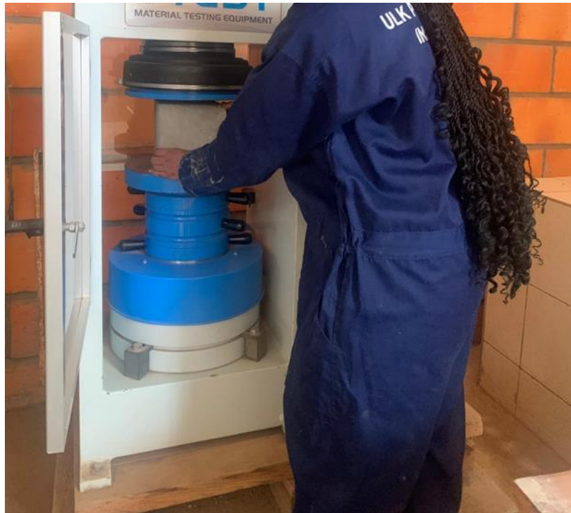
Figure 3. 11: Performing compressive strength test
