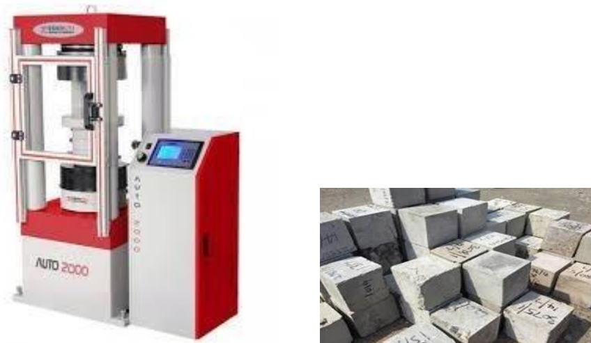
Figure 2. 9: Concrete cubes specimens and compressive machine
