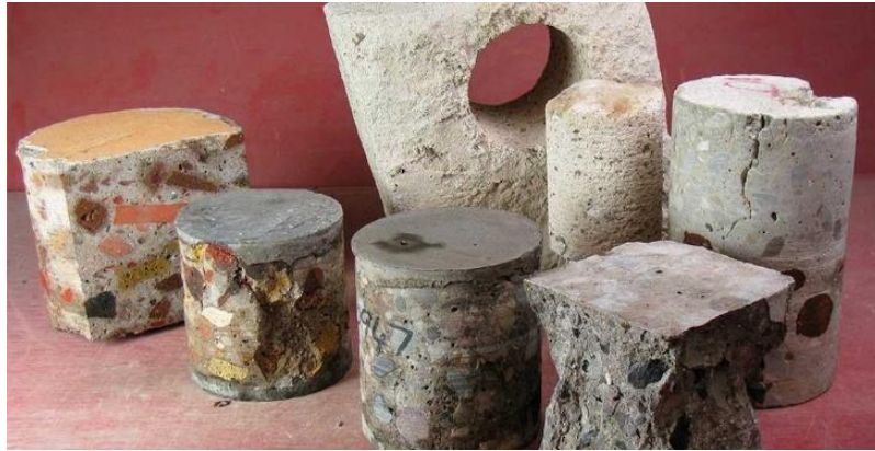
Figure 2. 8: Example of hardened concrete
