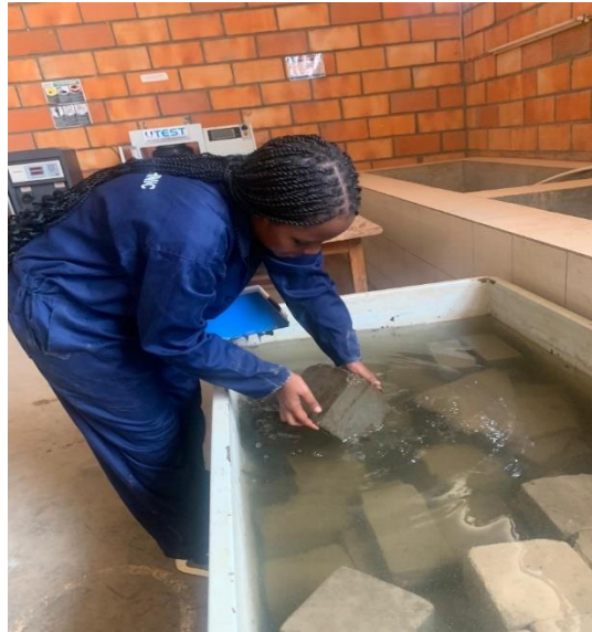
Figure 3. 10: during curing process
