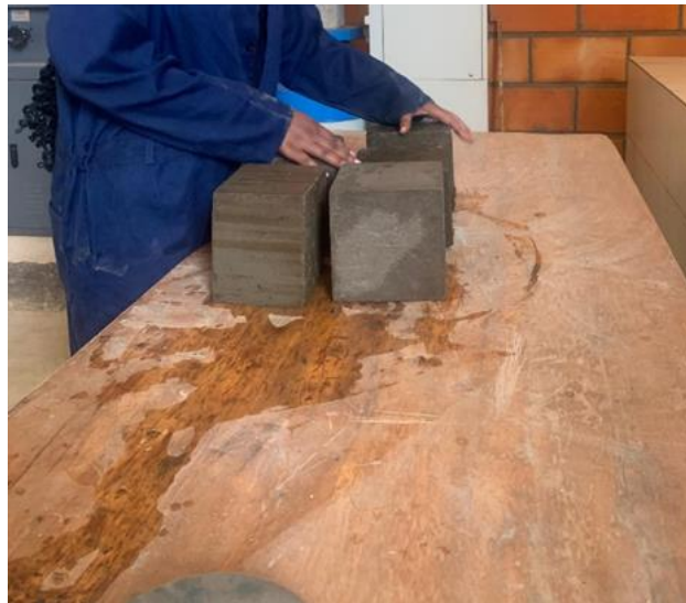
Figure 4. 1: Specimen boxes ready for test after curing
