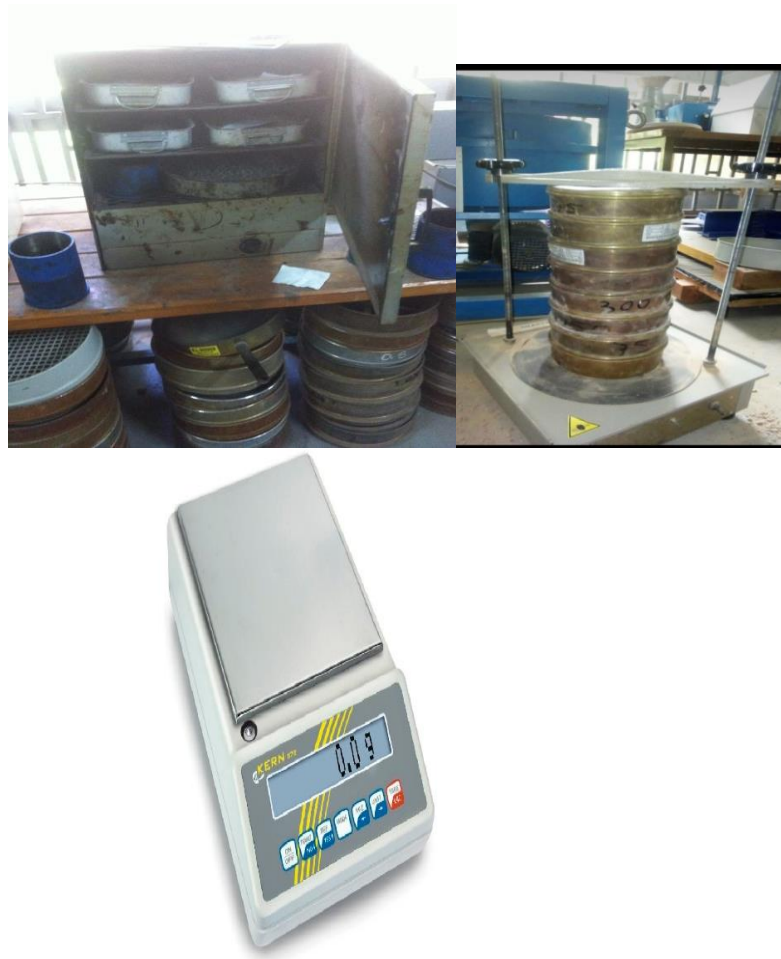
Figure.3. 7.shows the sieve sizes successively rest on the electrical shaker machine, balance and oven
