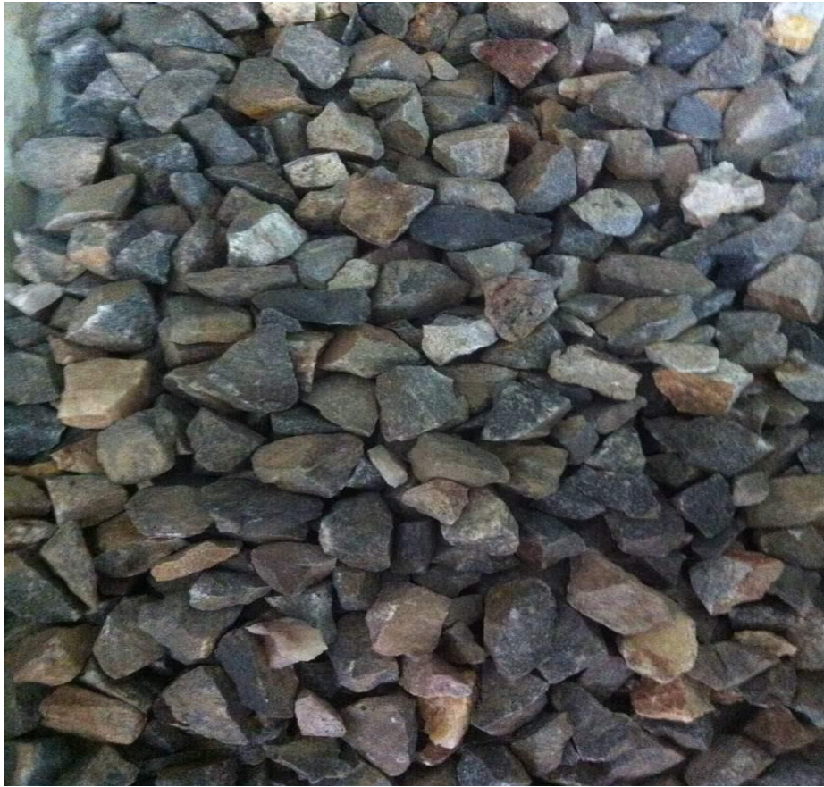
Figure.3. 3.Shows the crushed stone aggregates which will be used in the concrete cubes
