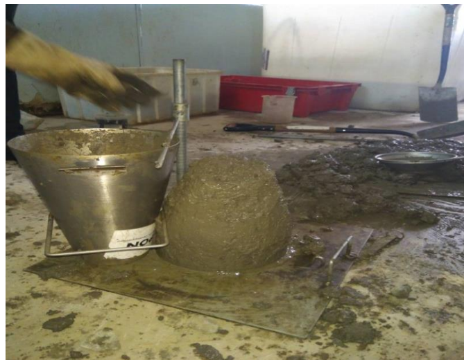
Figure.3. 10.shows the slump of the fresh concrete
