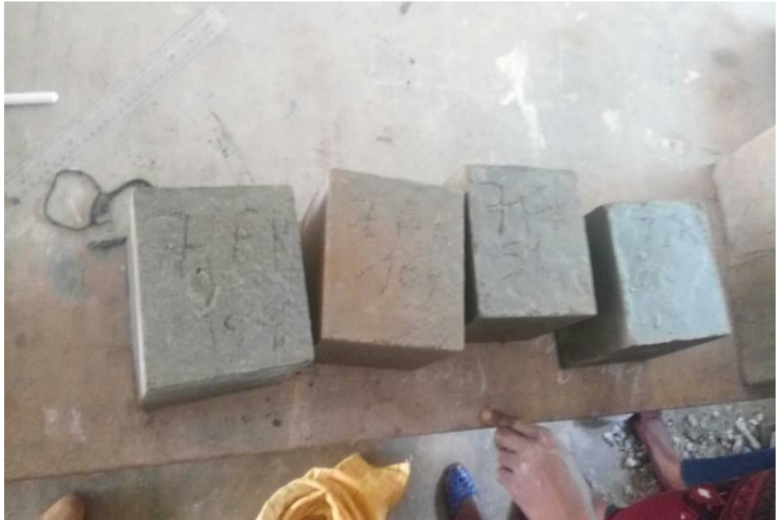
Figure.3. 12.show the cubes ready to be used in the compressive machine for 7 days test
