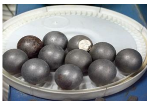
Figure.3. 8.different equipment used in los Angeles abrasion test such as steel balls, balance and abrasion machine.
