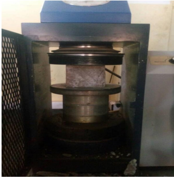
Figure.3. 13.Shows the concrete compressive machine and the cube rest on steel plates holding it ready to be crushed
