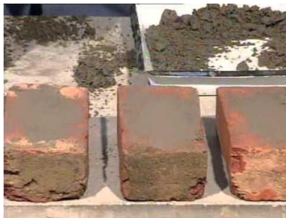
Figure 2.10: Frog portion of Brick filled with Cement Mortar
