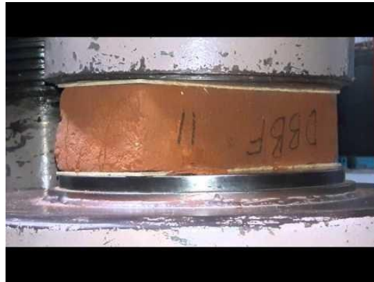
Figure 2.11: Compression test of a clay Brick specimen
