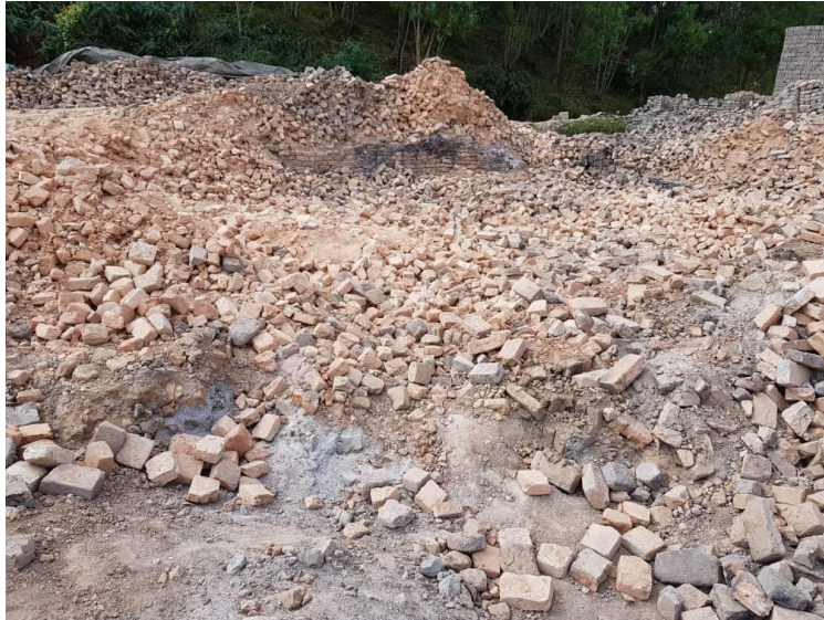
Figure 2.7: wastage of clay burnt bricks after burning them in clamp
