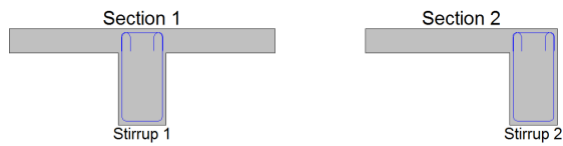
Figure 4. 21: Stirrups cross section
