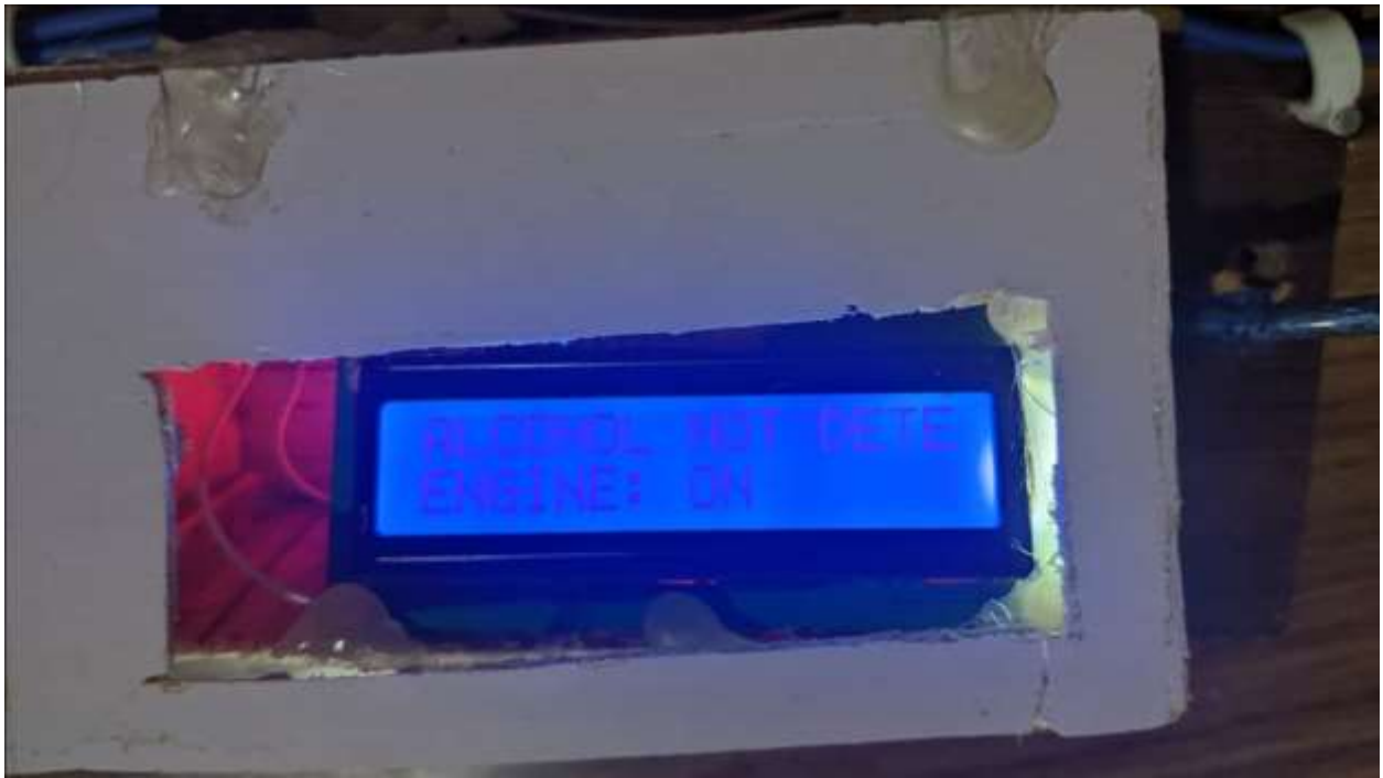
Figure 14: alcohol not detected Engine ON
