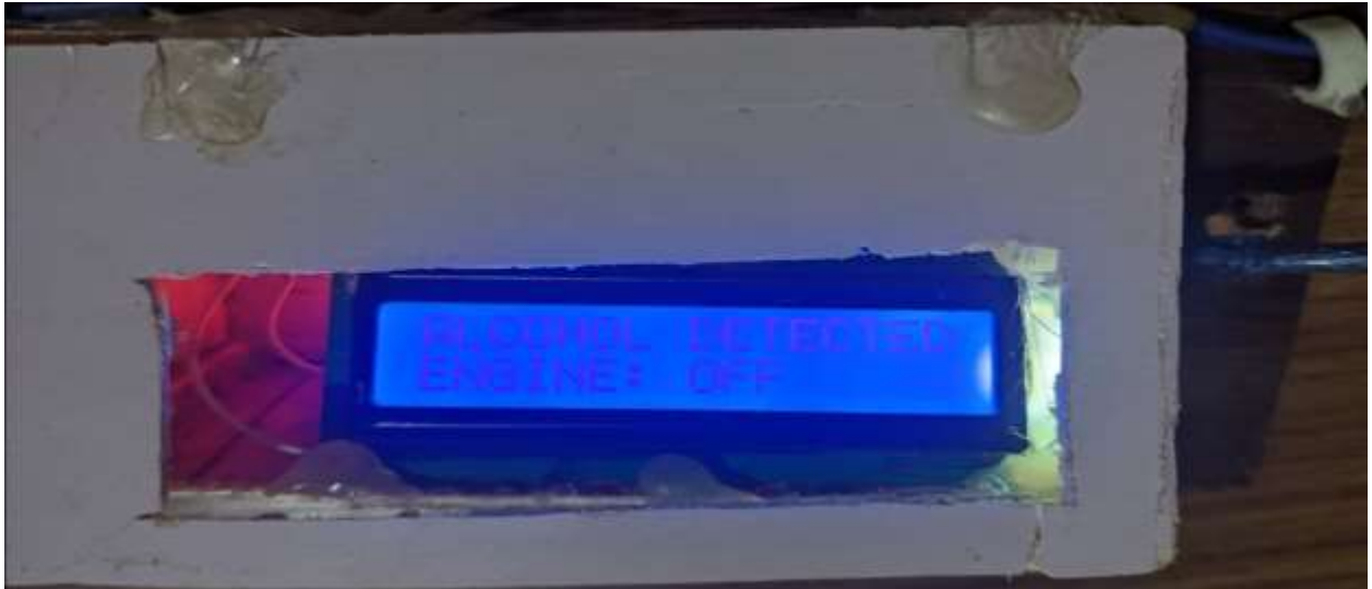
Figure 17: alcohol detected engine OFF
