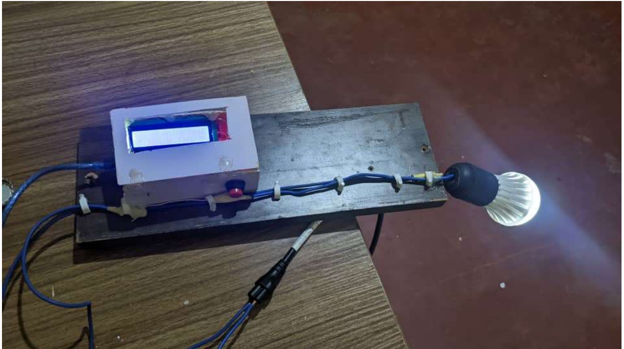
Figure 15: alcohol not detected engine indicator lamp ON
