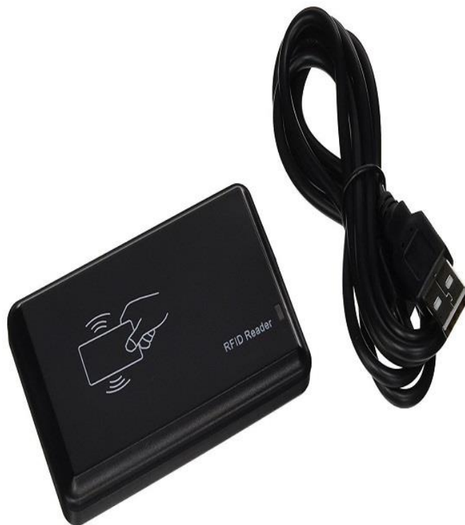
Figure 7 RFID scanner used to read unique identifiers from RFID cards to record attendance accurately.
