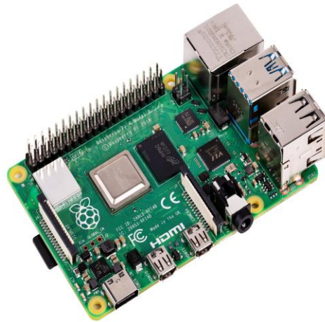
Figure 9 Raspberry Pi 4B, serving as the central processing unit for managing data and controlling hardware components in the RFID-based attendance system.
