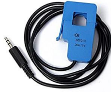
Figure 6. Current Transformer (Jadhav & Rajput, 2019)
